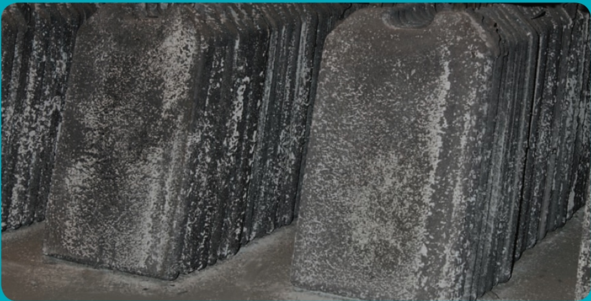
The molten material from the molds (above) cools and hardens into anodes containing 75% nickel. These are sent via narrow-gauge rail to the Refinery for processing into 99.9% pure nickel.
