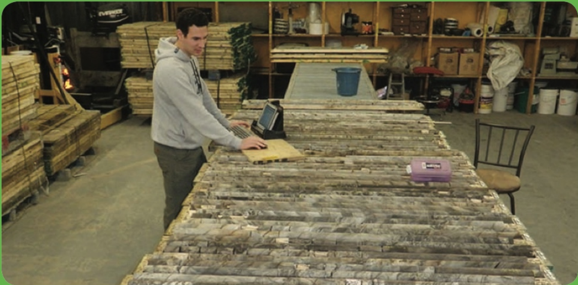
Diamond drilling produces thousands of meters of drill core each year. Drill core is visually analyzed, prepared for laboratory analysis, logged and catalogued. It is the foundation for mapping orebodies.
