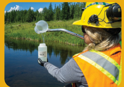
Collecting a water quality sample for the Weir final discharge point.
