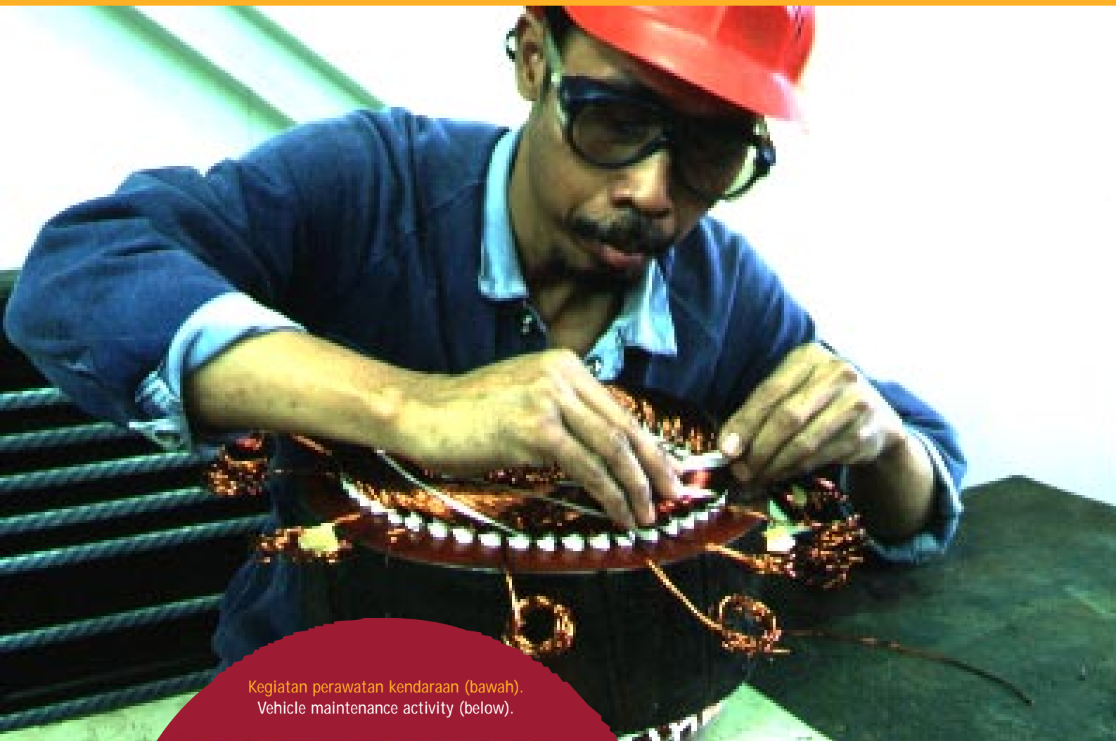
Abbas, teknisi, menggulung motor listrik di bengkel pusat pemeliharaan. Abbas, technician, rewinds an electric motor at the central maintenance workshop.
